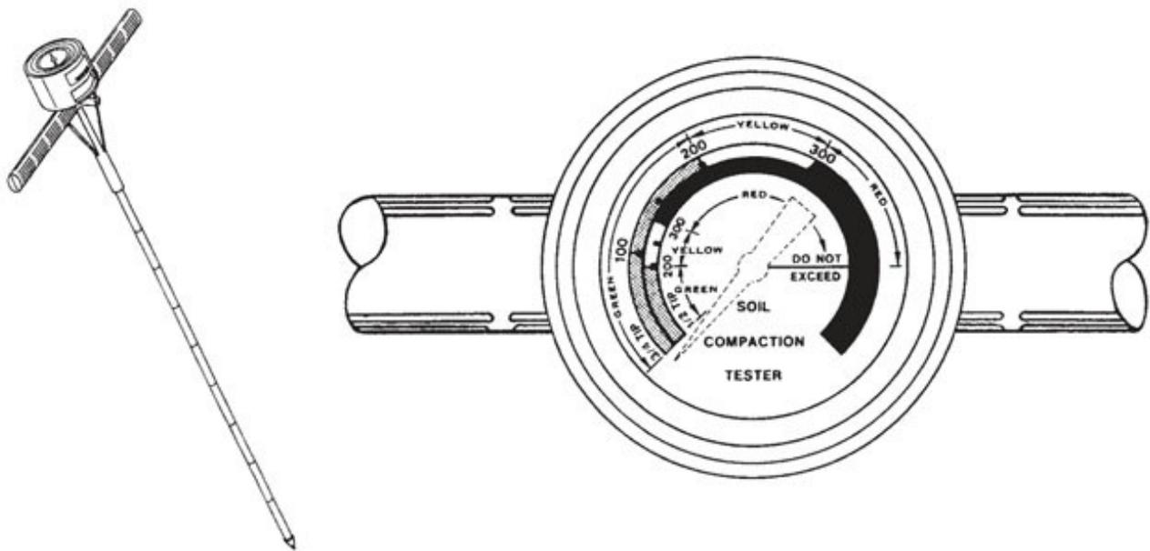
Figure 1a. A penetrometer, or soil compaction tester, has a graded shaft and separate reading scales for each tip. (Figure courtesy of Dickey John)
