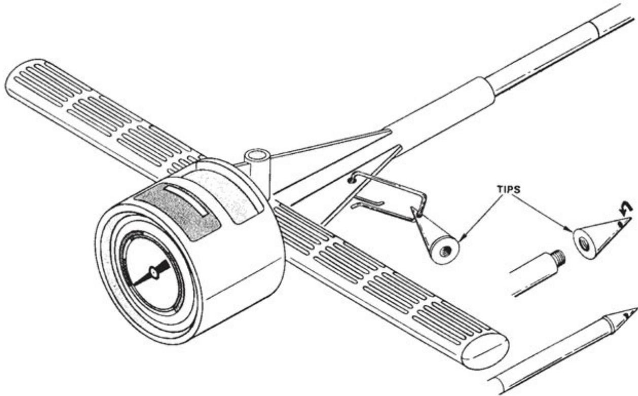
Figure 1b. A penetrometer usually comes with two points ( $\frac{1}{2}$  and  $\frac{3}{4}$  inch diameter). (Figure courtesy of Dickey John)
